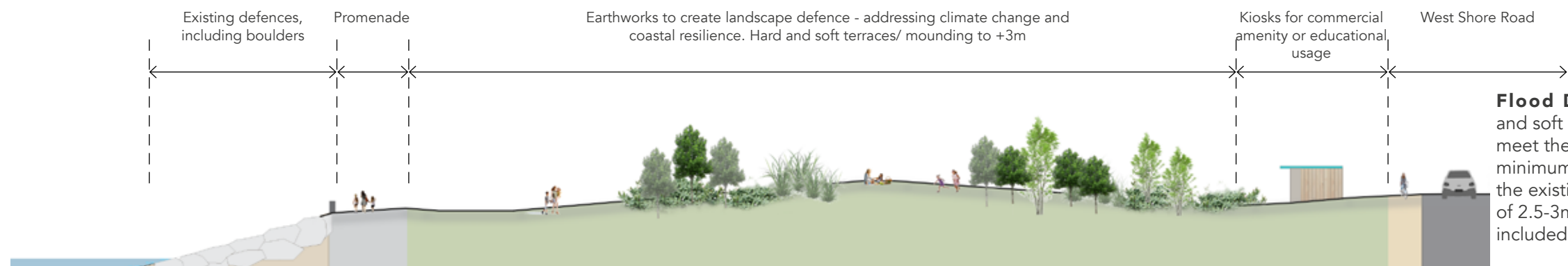
Fig. 5.3: Section A-A through flood defence landform, diagram by LUC Indicative proposal subject to consultation with HRA and SEA.
