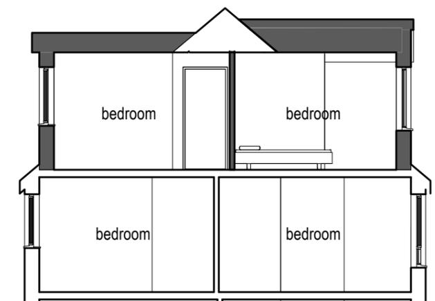
section a-a (first floor & attic floor)
