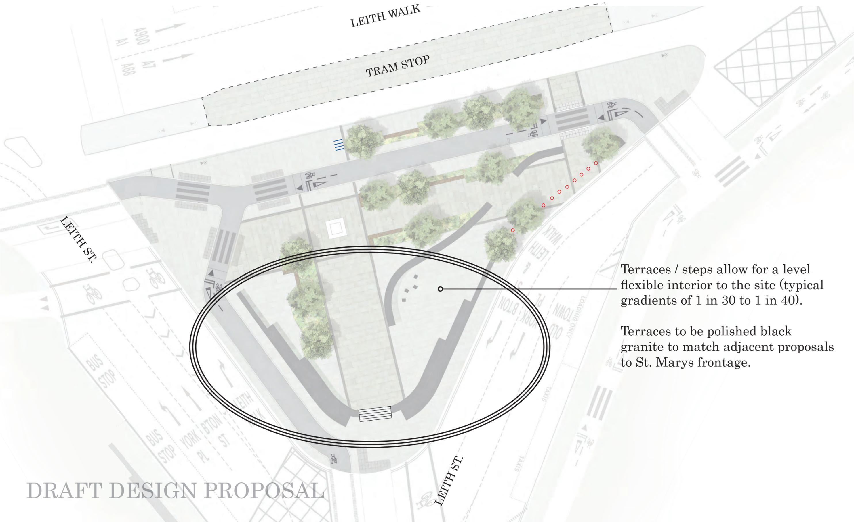
Terraces / steps allow for a level flexible interior to the site (typical gradients of 1 in 30 to 1 in 40).
