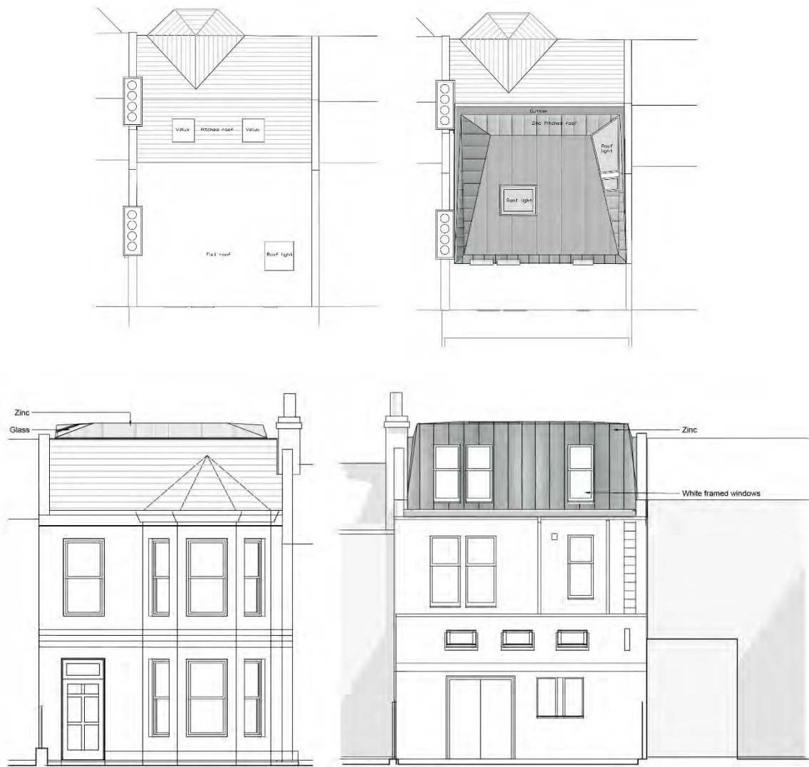
Figure 38 – Existing roof plan (top left), proposed roof plan (top right) and elevation proposals (below plans) for 20 Claremont Road
