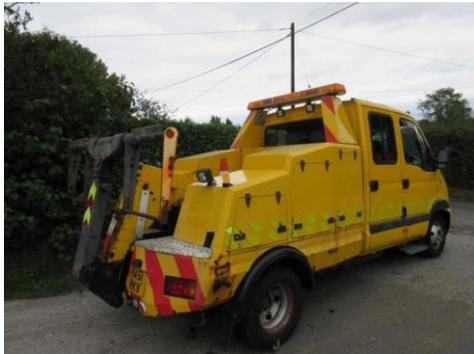
This approach generally involves a tow truck with a hydraulic rear lift that can be lowered to lift the front wheels of a vehicle off the road and tow it away.
