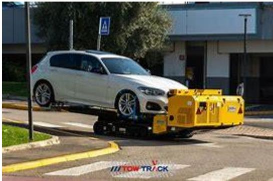
A third-party supplier can provide a Tow Track vehicle which is a remotely controlled and operated hydraulic lifting system, thus personnel are not in contact with lifting equipment and at risk should there be an electrical strike. The unit runs on tracks and uses hydraulics to completely lift a vehicle just two feet off the ground, essential for the recovery of electric and automatic vehicles. Thus, it potentially could safely work under the trams overhead power cables.
