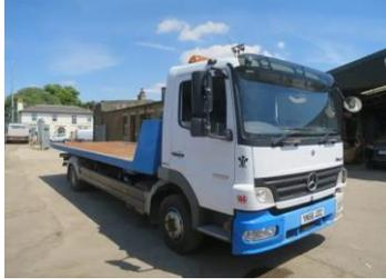
While this approach avoids a crane rising too close to the overhead power cables, vehicles would likely need to be dragged out of parking places, possibly at an angle, so that the vehicle can then be winched onto the flat bed of the truck.
